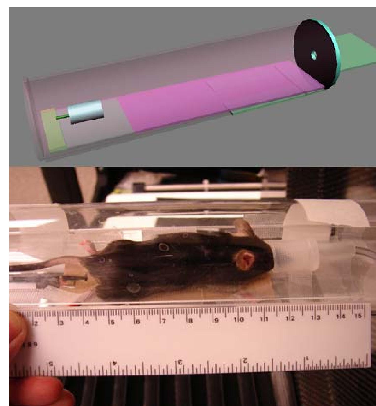
**Figure 2:** Imaging chamber that is compatible in microPET, CT and optical scanner.
