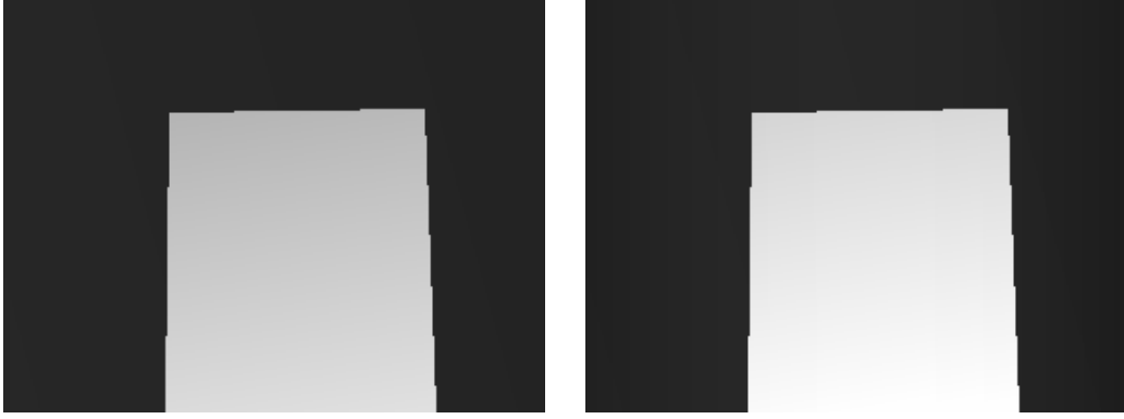
Figure 7.11 Disparity morphing result. The left image is original disparity map from an off-axis camera setup, and the right image is the generated disparity map for the toe-in camera setup with our conversion formula Eq. (7.17).
