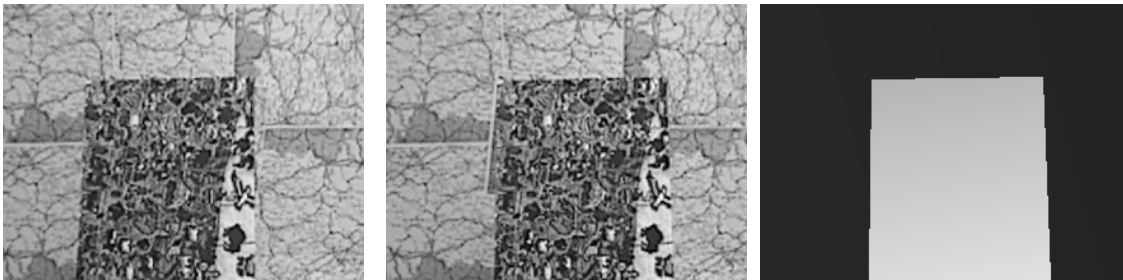
Figure 7.2 Sample stereo pair and its depth map. From left to the right are: left image, right image, the disparity map for the right image. The camera setup is off-axis, meaning that the optical axes of the left and right cameras are parallel.
