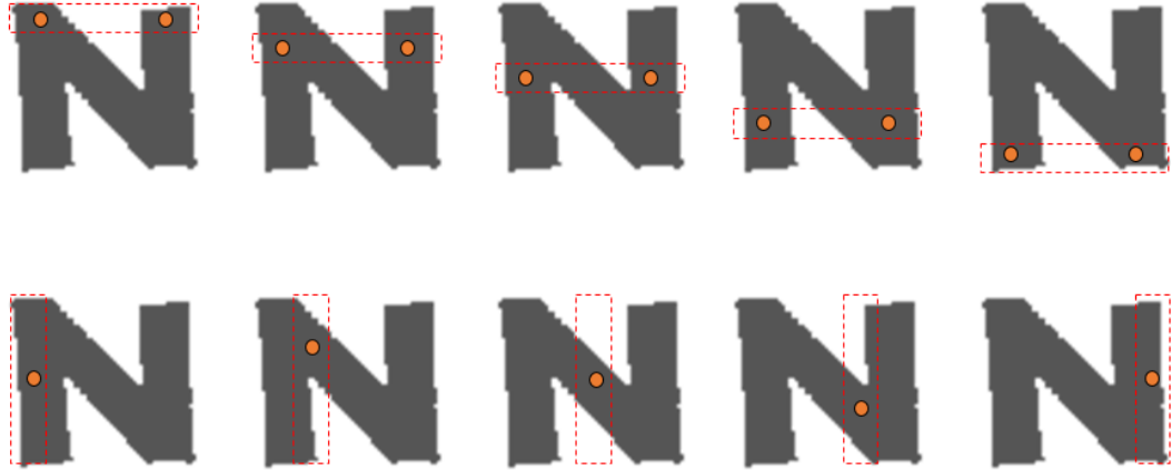
Figure 4.4: Stripe scan feature for text component using horizontal stripes (top row) and vertical stripes (bottom row). The example is for explanation purpose only. \tilde{v} = \tilde{h} = 5 , HSS = 0 and VSS = 0
