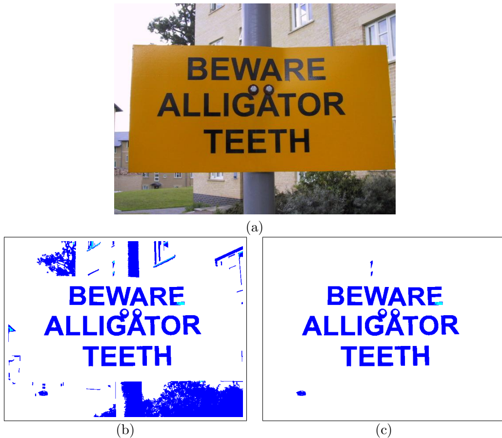
Figure 4.9: Geometric filtering (a) Sample image (b) Detected stable extremal regions (c) Output after geometric filtering
