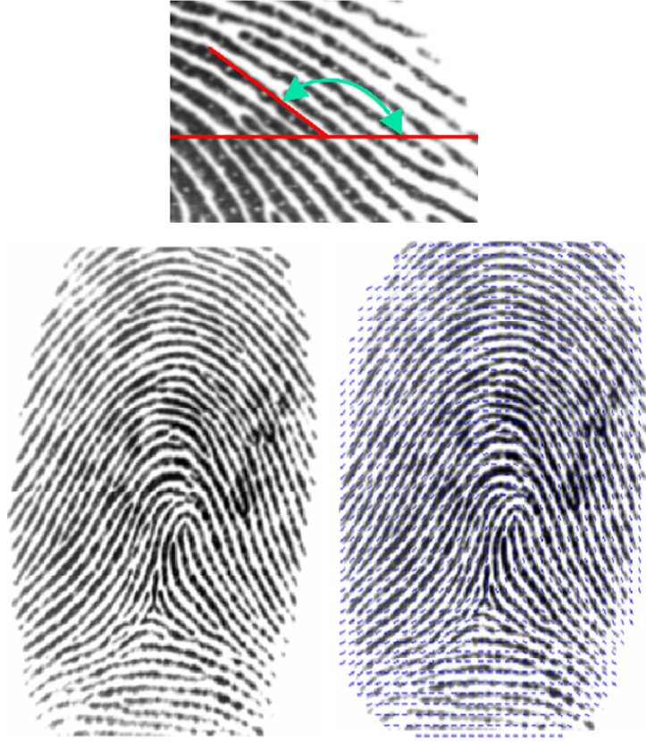
Figure 2.9: Definition illustration about orientation at fingerprint pixel and an orientation field estimated for an exemplary fingerprint. Blue lines means the estimated orientation in the local block. Image Credit: online resource.
