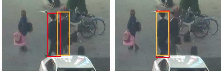
Figure 5.3: Illustration of the "jump-merge" tracking error, where the left image shows two correct tracking boxes for two similar targets in frame t - 1 and the right image shows the tracking result in frame t , where the yellow target region merges into the red target region resulting in an ID switch error.
