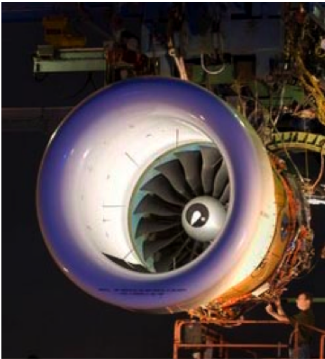
Figure A.3: PW4000 Engine - this picture shows a PW4062 engine as it appears on the test cell. The large add-on assembly seen in front of the fan includes sensors and instrumentation used for the collection of high fidelity data streams. The engine can be seen mounted at a test cell facility. Some of these facilities allow for the simulation of high altitude temperature and pressure conditions, though most measure engine operation within local ambient conditions that are referenced to earlier baseline recordings. (photo courtesy of UTC Pratt-Whitney)
