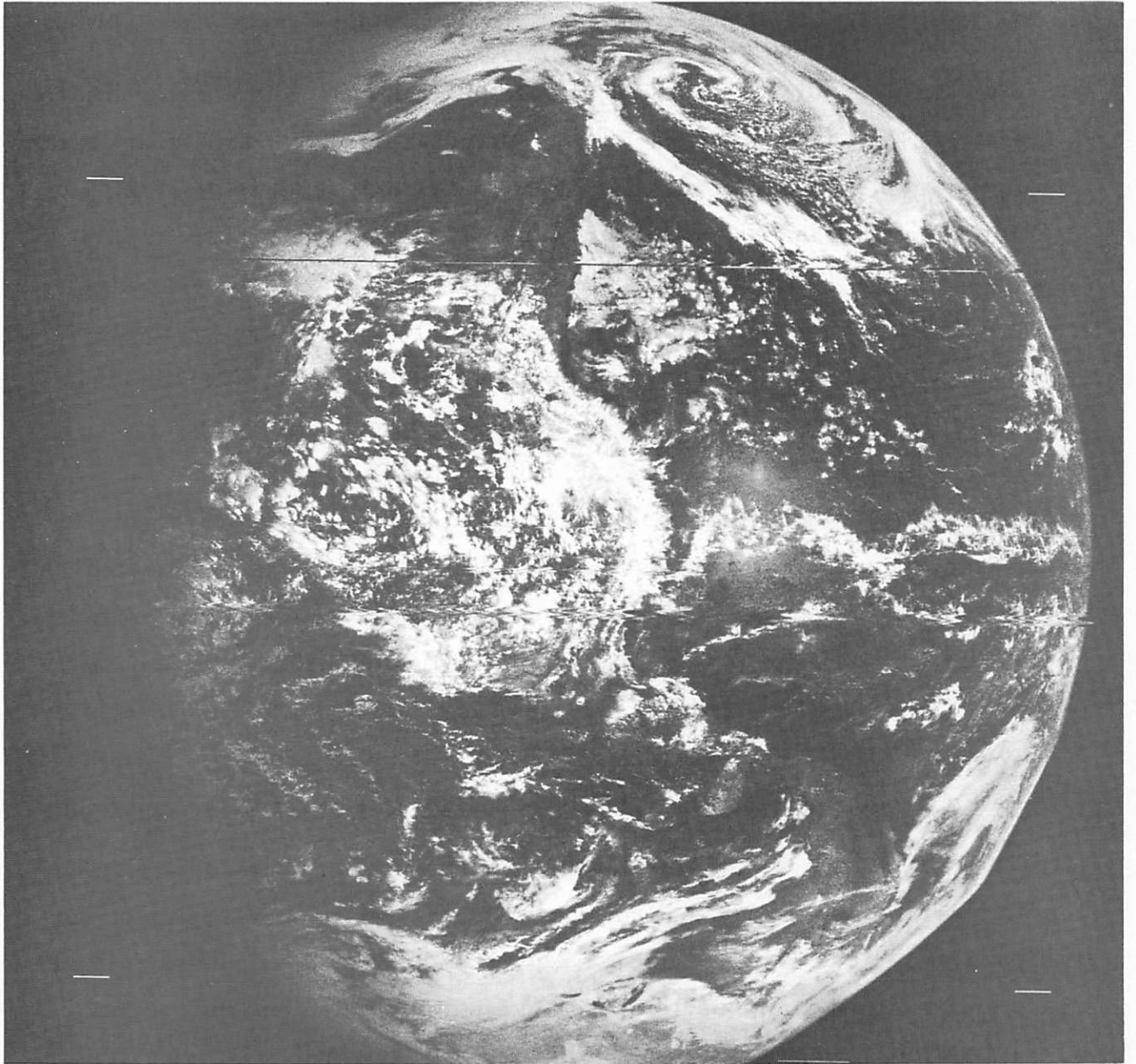
Figure 3.1-1. Compressed ATS colored picture using information preserving coding of pixel differences - 3.0 bits/pixel.
