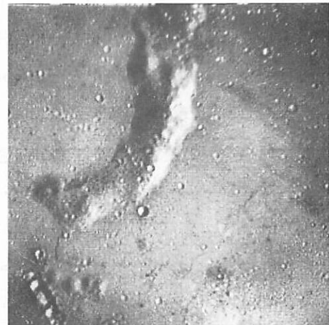
(f) Image processed by Gaussian isotropic high frequency emphasis filter followed by histogram equalization.
