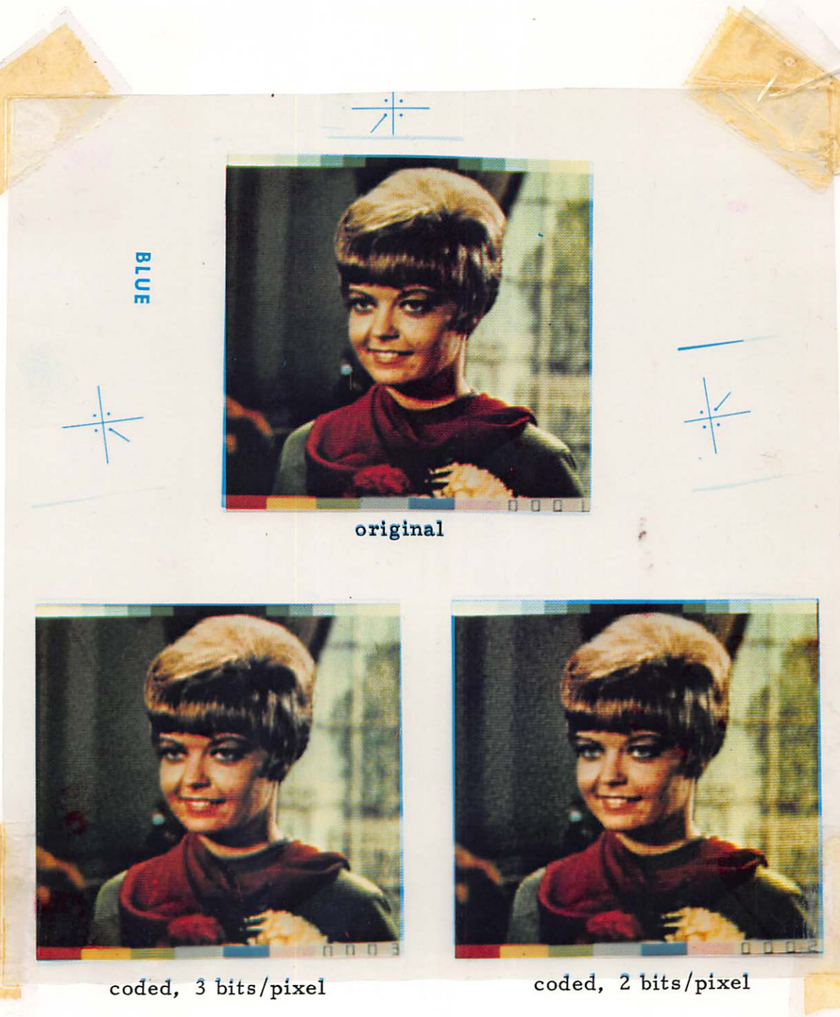
Figure 3.1-4. Original color image and coded reconstructions for Slant transform color image coding.
