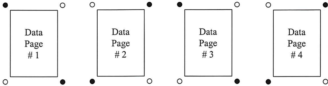
Figure 8.2 An example of the data page tracking in a two-photon PODS system with four clock channels at each corner of a data page (each filled circle represents a data mark or a “1” bit).
