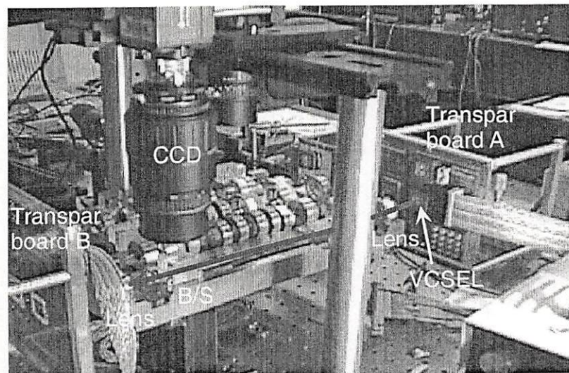
Figure 5-3. Picture of free-space optical interconnection experiment setup.
