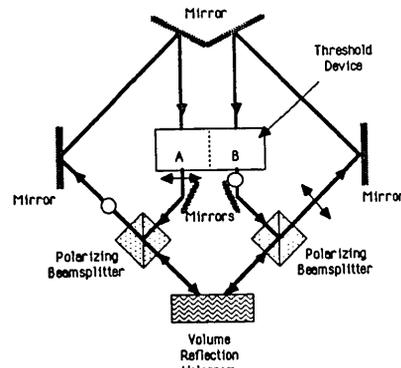
Fig. 3. BAM volume reflection hologram.
