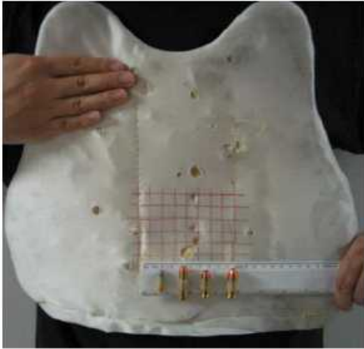
Fig. 2. One of the authors holds a 14-ply Kevlar soft body armor panel (from a Superfeatherlite vest from Second Chance) and some sample cartridges (.22, .38, .40, and .45 caliber). Different caliber bullets struck the sample armor but did not include a .44 caliber.
