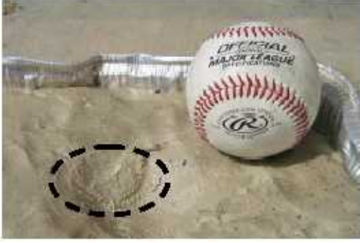
Fig. 7. A regulation baseball and a record of its impact. Pitching machines threw baseballs at tubs of plumber's putty. A chronograph measured the speed of each baseball. The baseball speeds were approximately 40, 50, 60, 70, 80, and 90 miles per hour.
