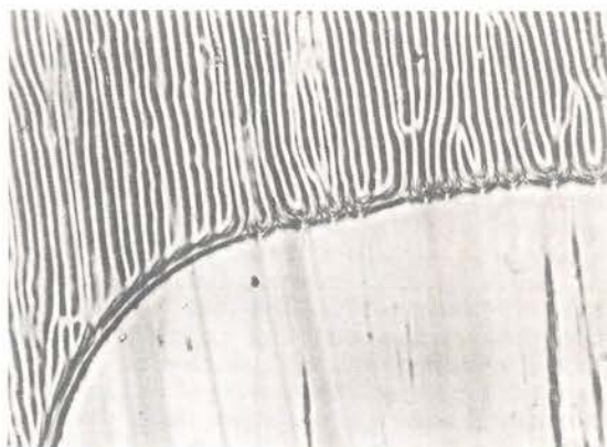
Figure 7. Behavior of domains near an edge. Magnification 100 times.
