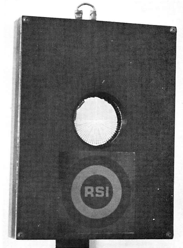
(b) ring and wedge detector assembly.
