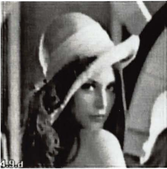
(c) The rsetored image using the modified MMSE filter.
