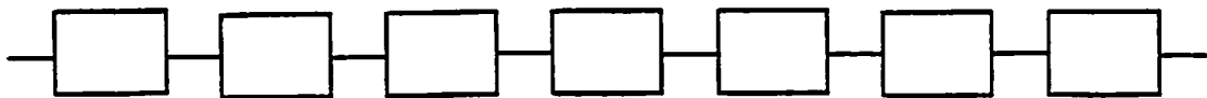
Figure 2.2: A cellular string. It requires only a 1-D interconnection geometry. Each cell only connects with its two nearest cells.
