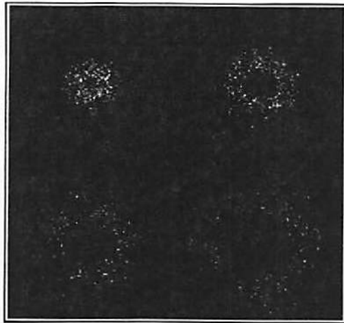
Figure 7.15 Four data images collected from a single Ge detector at four different Compton scattering angles.
