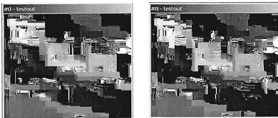
Figure 2.7: (a) Frame no. 1 and (b) frame no. 9 of the RHT-encrypted "Foreman" video clip decoded using the standard H.264 decoder
