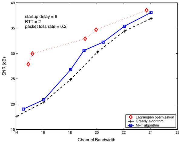
**Figure 4.** The comparison of SNR under different scheduling algorithms with various channel bandwidths. (Lagrangian algorithm:  $N = 12$ . M-T algorithm:  $M = 8, T = 8$ .)
