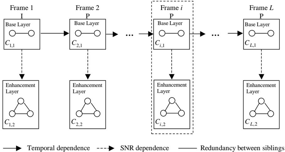
**Figure 2.** An example DAHG of the MDLC system for a group of I-P frames.
