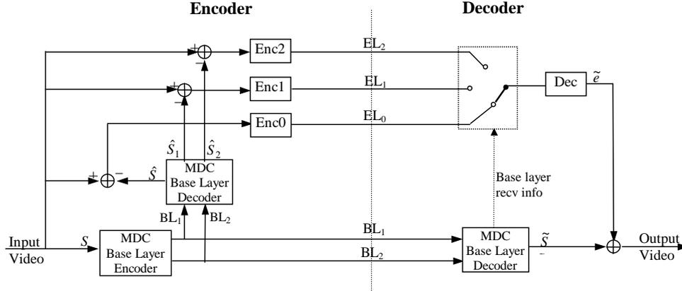
Figure 1. Structure of the MDLC codec.
