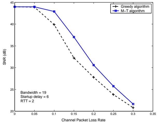
**Figure 5.** The comparison of SNR under different scheduling algorithms with various channel packet loss rates. (M-T algorithm:  $M = 8, T = 8$ )
