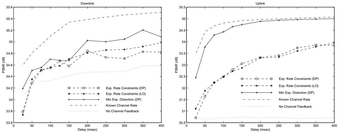
Fig. 10. **Two-state Markov channel model:** Resulting PSNR of the decoded video under end-to-end delay constraint from 50 msec to 400 msec. Dynamic Programming (DP) and Lagrangian Optimization (LO) are used for selecting encoding rates.
