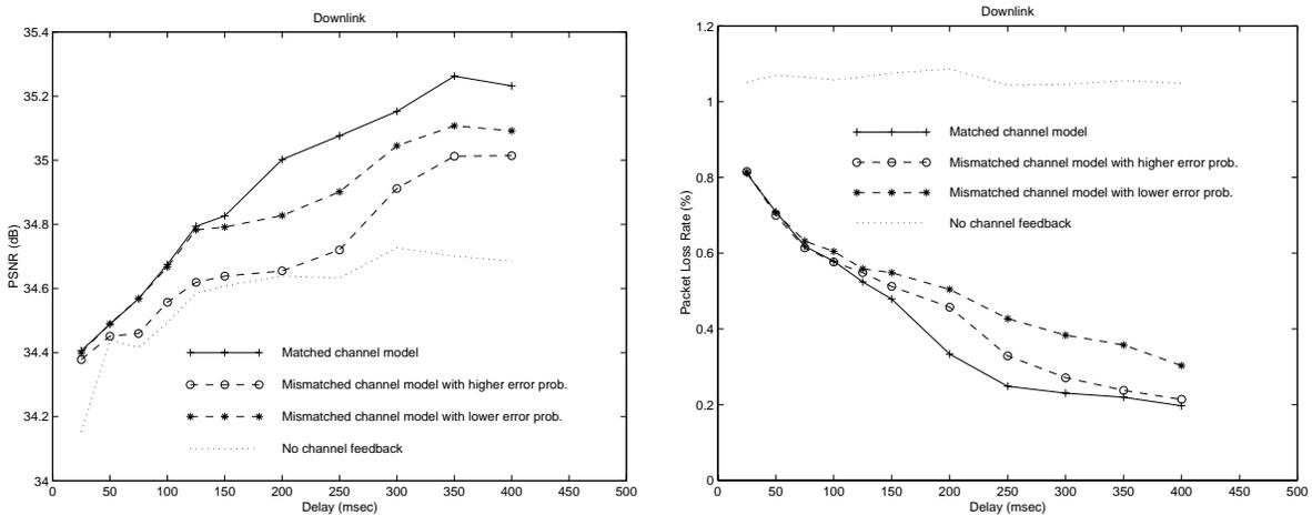
Fig. 14. **Mismatched Channel Models:** Resulting PSNR and packet loss rate of the decoded video when inaccurate channel models are used. Rate control is based on dynamic programming approach to minimize expected distortion.
