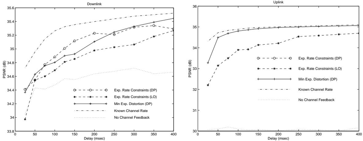
Fig. 8.  $N$ -state Markov channel model: Resulting PSNR of the decoded video under end-to-end delay constraint from 50 msec to 400 msec. Dynamic Programming (DP) and Lagrangian Optimization (LO) are used for selecting encoding rates.
