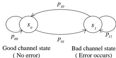
Fig. 5. Two state Markov channel model.
