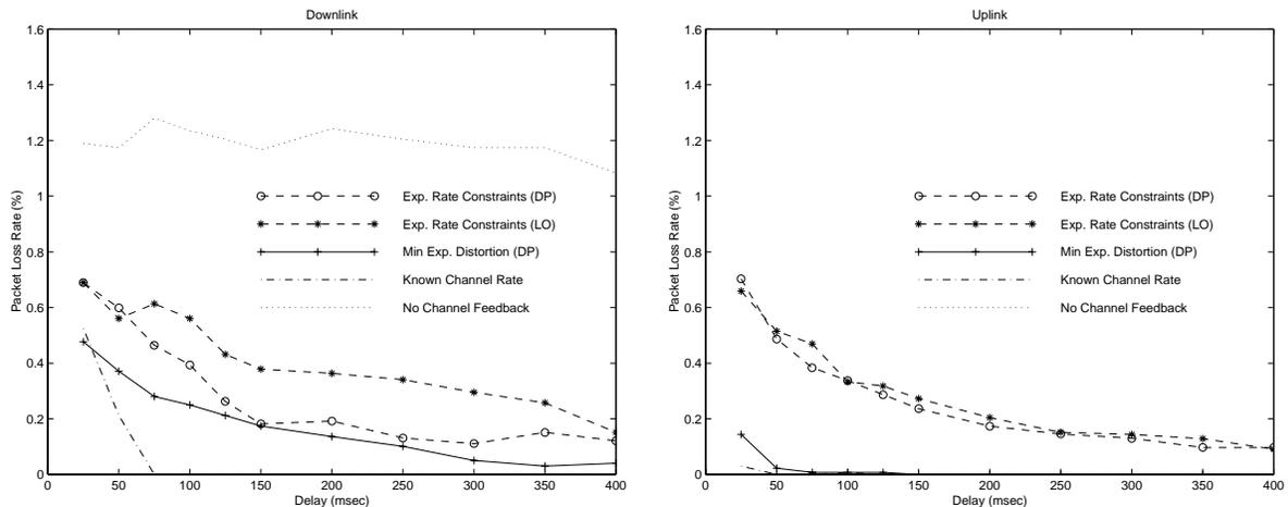
Fig. 9.  $N$ -state Markov channel model: Resulting packet loss rate under end-to-end delay constraint from 50 msec to 400 msec. Dynamic programming approach with minimal expected distortion criteria is used as rate-control algorithm.
