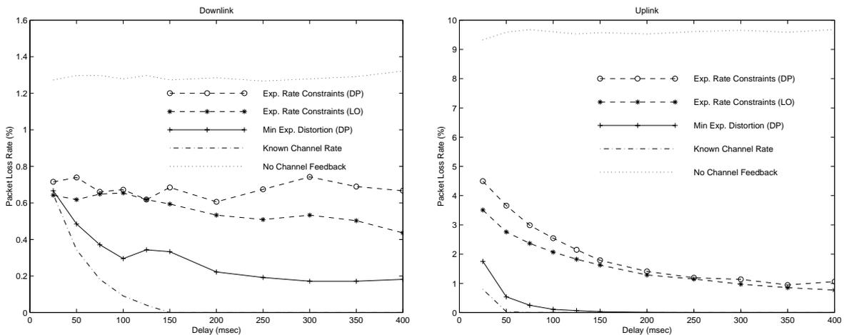
Fig. 11. **Two-state Markov channel model:** Resulting packet loss rate under end-to-end delay constraint from 50 msec to 400 msec. Dynamic programming approach with minimal expected distortion criteria is used as rate-control algorithm.
