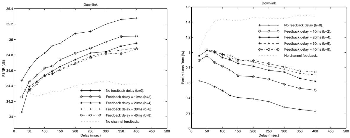
Fig. 13. **Performance Degradation Due to Feedback Delay:** Resulting PSNR and packet loss rate of the decoded video with various feedback delays. Rate control is based on Lagrangian optimization approach with expected rate constraints.
