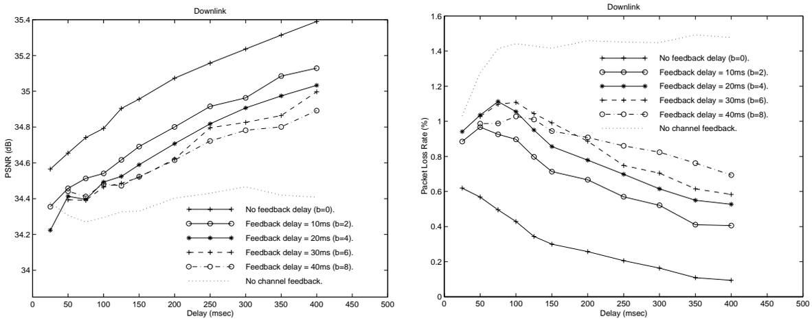
Fig. 12. **Performance Degradation Due to Feedback Delay:** Resulting PSNR and packet loss rate of the decoded video with various feedback delays. Rate control is based on dynamic programming approach to minimize expected distortion.
