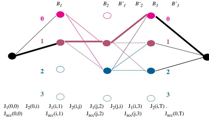
Fig. 5. A heuristic fast search. The trellis in Figure 4 can be restricted using the proposed fast search algorithm. The underlying assumption is that the reference image is more important than the difference. The search space is reduced to the nodes selected by the blockwise quantization for the reference image.
