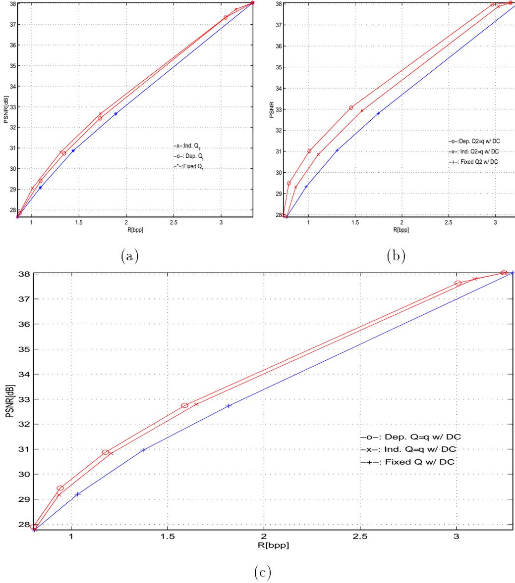
Fig. 8. RD performance comparison. (fruit.256, Block size= $8 \times 8$ ,  $SW = 10$ ,  $|Q| = 8$ ,  $QS = \{90, 80, \dots, 20\}$  and  $\lambda = \{0, 0.1, 0.5, 1, 2, 100\}$ ). The points marked with + correspond to the results of JPEG with DC. The points marked with  $x$  and  $o$  correspond to blockwise independent and dependent QS selections, respectively. RD characteristics for (a) the reference image, (b) the DCD frame, and (c) the two images.
