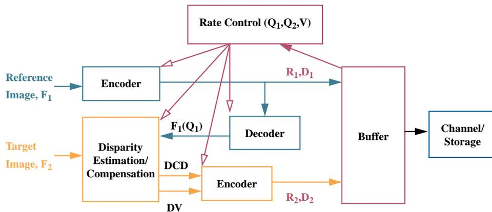
Fig. 1. Block diagram of a general encoder for stereo images, where encoder consists of disparity estimation/compensation, transform/quantization and entropy coding.
