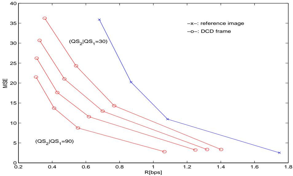
Fig. 9. Mean ORD plots for the block in the reference image and the DCD frame. (room.256,  $QS = \{90, 70, 50, 30\}$ )  $QS_2$  is changed for the DCD frame with a given  $QS_1$ . As shown, the monotonicity property is satisfied, i.e.  $J(QS_2|QS_1^*) \leq J(QS_2|QS_1)$ , for  $QS_1^* \geq QS_1$ . In particular, if  $\lambda = 0$ ,  $d(QS_2|QS_1^*) \leq d(QS_2|QS_1)$ , for  $QS_1^* \geq QS_1$ .
