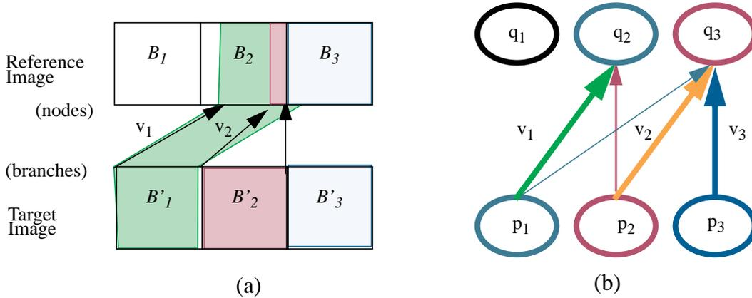
Fig. 3. Binocular dependency between corresponding blocks along the disparity vector. At most two consecutive blocks in the reference image are related to a block in the target image. For example, a block  $B'_1$  in the target image is compensated from (at most) two consecutive blocks,  $B_2$  and  $B_3$ , in the reference image along the disparity vector  $v_1$ . Therefore, the distortion of the block in the DCD frame is a function of  $p_1$ ,  $q_2$  and  $q_3$ .
