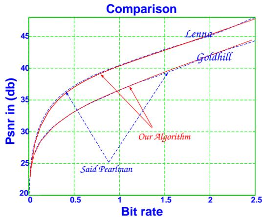
**Figure 4. Rate Distortion Curves for the  $512 \times 512$  Lenna and Goldhill images. Comparison between our algorithm and [2]**
