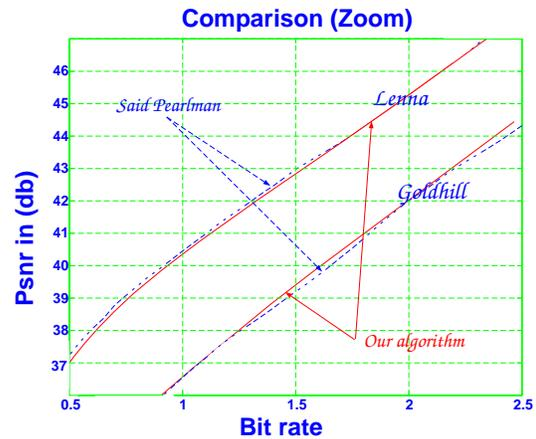
**Figure 5. Rate Distortion Curves for the  $512 \times 512$  Lenna and Goldhill images. Comparison between our algorithm and [2]**
