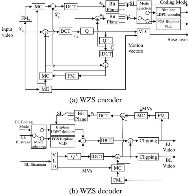
**Fig. 2.** The block diagram of WZS encoder and decoder. FM: frame memory, ME: motion estimation, MC: motion compensation.
