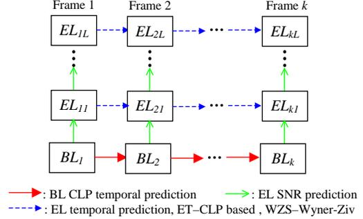
**Fig. 1.** Basic difference of prediction techniques used in ET and in proposed WZS.  $BL_i$ : the base layer of the  $i$ th frame.  $EL_{ij}$ : the  $j$ th EL of the  $i$ th frame, where the most significant EL bitplane is denoted by  $j = 1$ .
