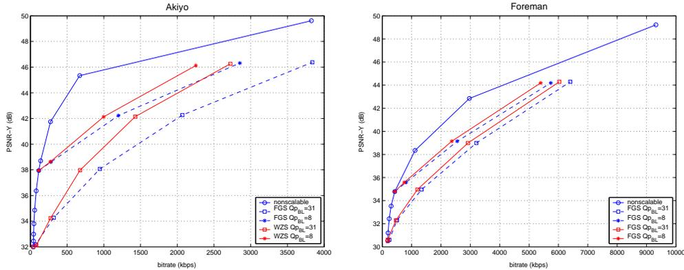
Fig. 4. Comparison between the proposed WZS, MPEG-4 FGS and nonscalable coding.
