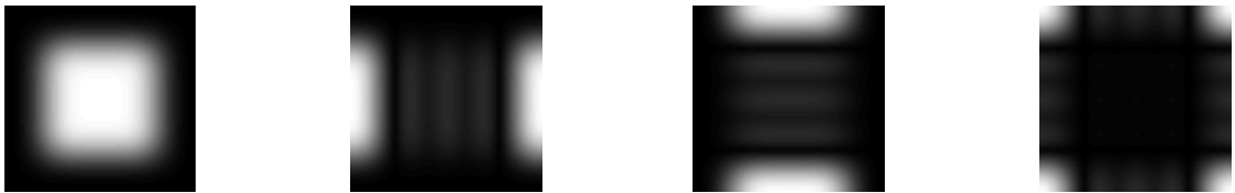
Figure 4.1: Set of 2D filters obtained from the 1D Daubechies orthogonal filter bank 'daub3'
