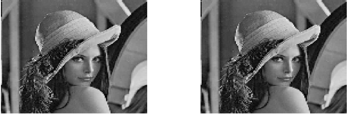
Figure 3.5: Lenna image coded using MDC-PT. Description 1 MSE = 22.16, Description 2 MSE= 22.01, Total Bpp= 1.79, HR MSE= 14.39, MSE is w.r.t. original image.
