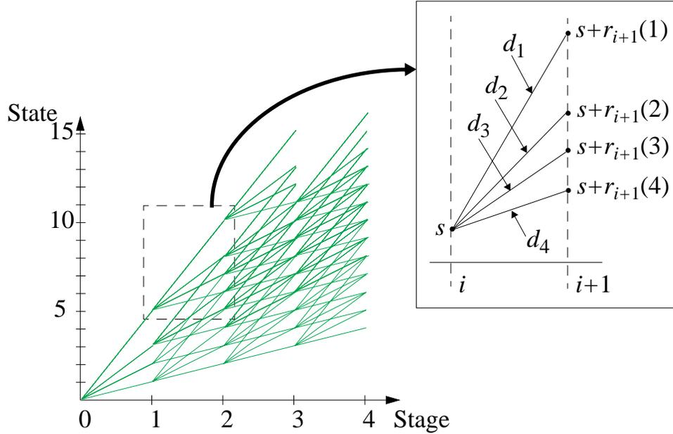
Figure 1.6: Components of the dynamic programming tree.
