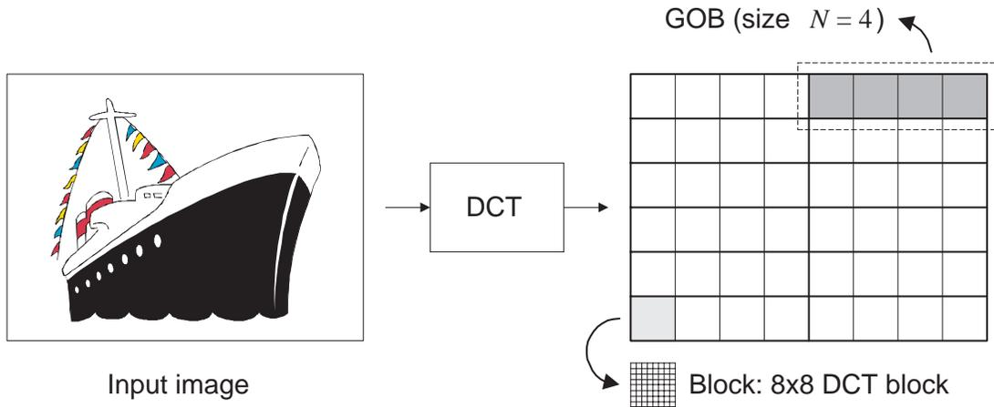
Figure 6.3: Definitions for our constant GOB rate coding. A *block* is an  $8 \times 8$  DCT block and a *group of blocks* (GOB) is a set of consecutive blocks over which the rate constraint is imposed. The GOB size ( $N$ ) is the number of blocks in a GOB.
