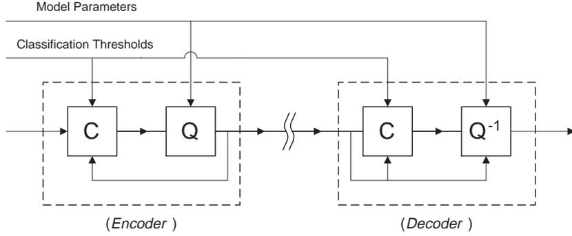
Figure 3.6: Overhead usage to help the backward adaptive classification scheme. The resulting overhead is negligible compared to those of forward adaptive block-based classification/quantization schemes.
