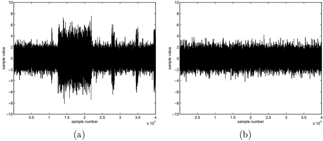
Figure 2.4: (a) Samples generated by a bimodal Gaussian source switching between two Gaussian sources,  $N(0,1^2)$  and  $N(0,2^2)$  with the transition probability 0.001. (b) Samples from  $N(0,1^2)$ .
