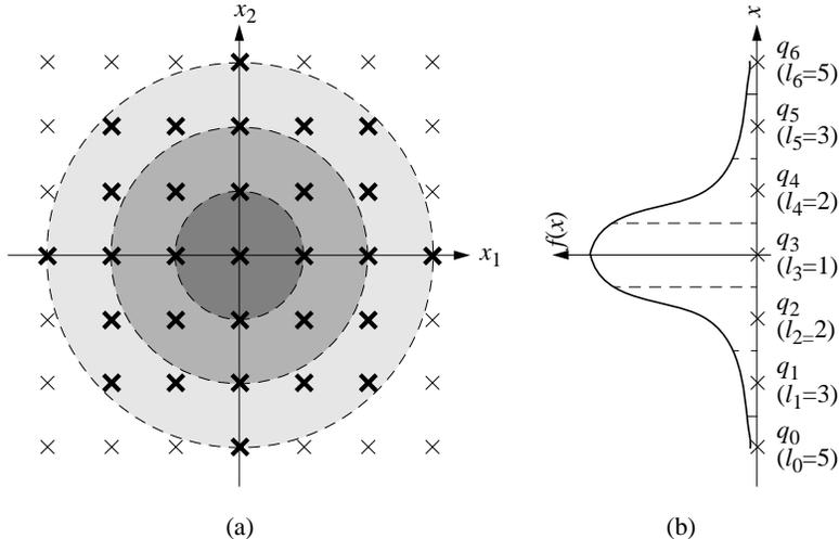
Figure 2.2: A 2-dimensional SVQ codebook derived from USQ for an i.i.d. Gaussian source. (a) SVQ codevectors are chosen from the 2-dimensional grid such that the codeword length is no greater than a pre-determined threshold  $L$ . (b) Quantization levels and the associated lengths of the USQ which determines each component of the vector grid.
