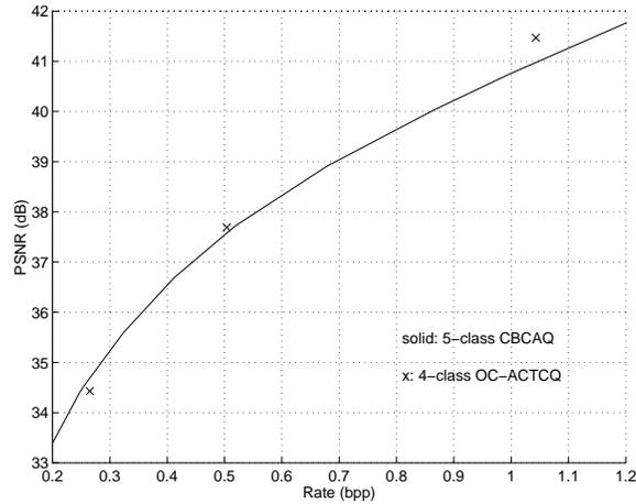
Figure 3.11: Comparison of two classification-based image coders, PC-AUTQ and OC-ACTCQ for Lena.
