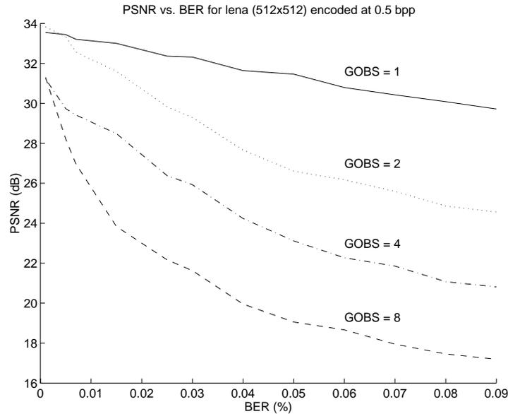
Figure 6.5: PSNR vs. BER obtained by the proposed scheme for various GOB sizes. The Lena image (512x512) is encoded at the target rate of 0.5 bpp for each simulation. The error robustness of the coding scheme yields graceful degradation of PSNR with worsening channel conditions and the small GOB sizes are particularly useful at high BERs.
