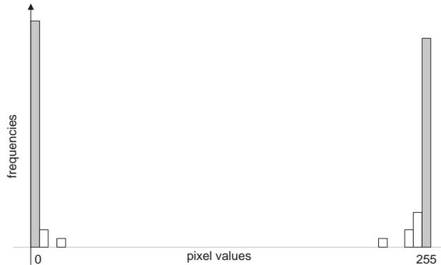
Figure 4.1: The histogram of a simple image is characterized by a few strong modes. The example shown here is a typical histogram of an 8-bit gray-scale image scanned from a bi-level image. While most pixel intensity values are either 0 or 255 (corresponding respectively to black or white pixels in the bi-level image), the scanning noise can cause a small number of pixels to have intensity values slightly different from 0 or 255.
