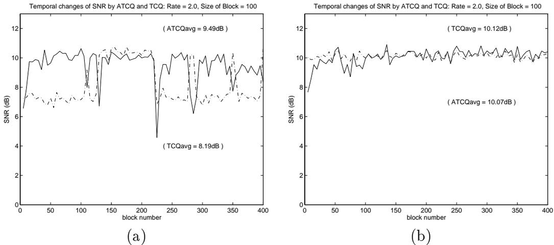
Figure 2.6: ATCQ vs. TCQ (a) When the input is bimodal, the performance of the ATCQ remains nearly constant throughout the sequence except at the point of mode change and outperforms the TCQ while the TCQ performance is better for one of the two modes. (b) For a stationary memoryless Gaussian input source, the ATCQ experiences a slight degradation in performance due to the adaptation.
