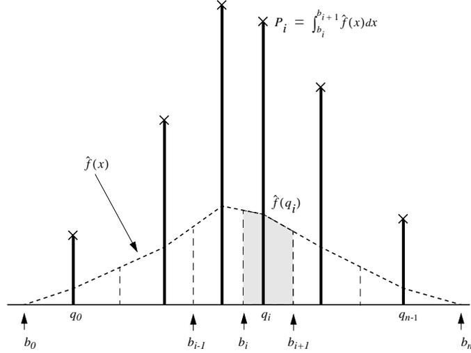
Figure 1.3: Input pdf estimation from histogram of past quantized data.
