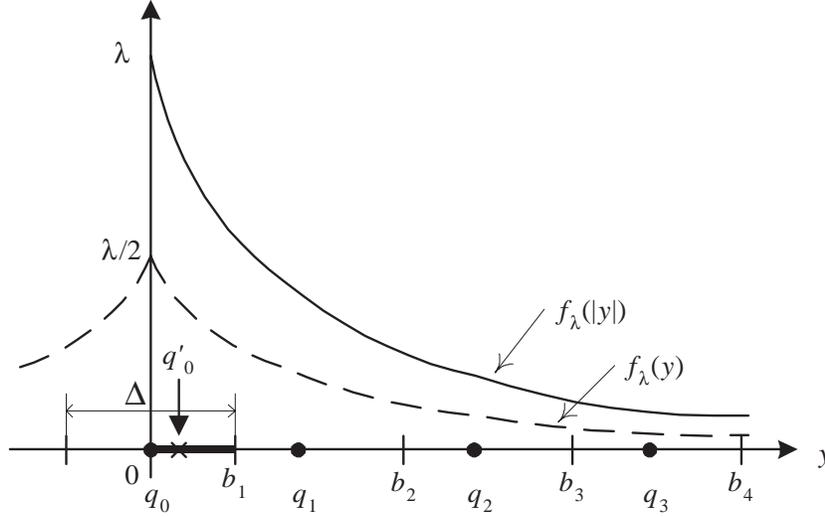
Figure 3.8: The positive half of the UTQ with stepsize  $\Delta$ .  $q_j$ 's and  $b_j$ 's are quantization levels and bin boundaries, respectively.  $q'_0$  is the conditional mean of  $|y|$ , i.e., the centroid, in the interval of  $[0, b_1)$  where  $|y|$  follows the exponential distribution  $f_\lambda(|y|)$ .
