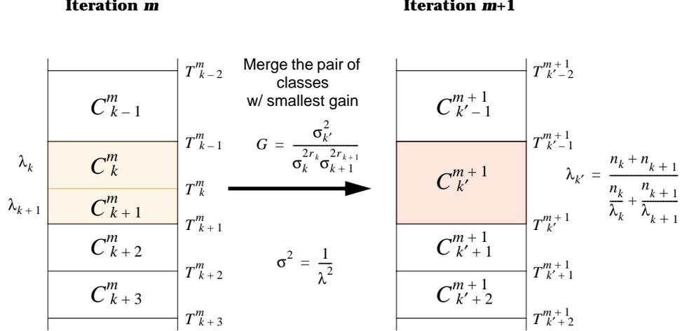
Figure 3.7: Illustration of the merging process in the classification threshold design. At the  $m$ -th iteration, the pair of the  $k$ -th and the  $(k + 1)$ -st classes has the smallest classification gain so as to merge into one class.
