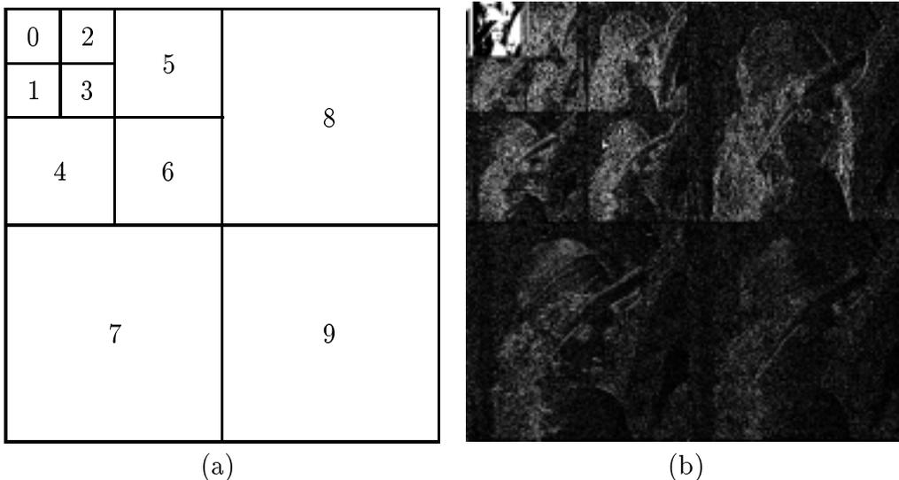
Figure 3.2: (a) Layout of the image subbands, with subband indices, from 3-level dyadic decomposition. (b) Subband coefficients obtained by 3-level dyadic decomposition of the Lena image using a wavelet filter set. We can observe frequency compaction of energy towards low frequency subbands and, more importantly, spatial clustering of the transform coefficients at similar energy level within each subband.
