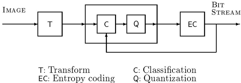
Figure 3.1: Building blocks in the conventional encoder for transform image compression. In our work the quantization block combines backward adaptive quantization and classification.
