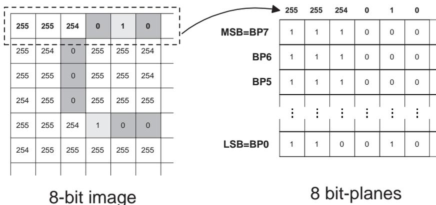
Figure 4.3: Bit-planes obtained from an 8-bit gray-scale image. In this figure one line of pixels in the image is converted into bit-planes.
