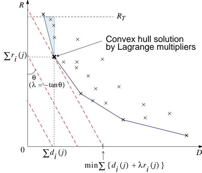
Figure 1.5: Lagrangian solution in the discrete R-D space. Lagrangian solutions are limited to the only convex hull points in the space of operating points. Note that the shaded area contains better solutions, including the optimal solution, in the sense they have smaller distortion than the convex hull solution still within the budget.
