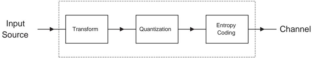
Figure 1.1: Block diagram of a generic encoding system.
