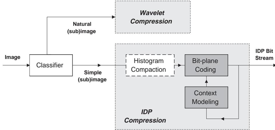
Figure 4.2: The block diagram of a generic coding system that can be consistently good for both natural and simple images. The Classifier block can be further generalized by assuming a segmentation function for the input image into natural and simple regions.
