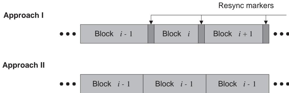
Figure 6.2: Bit streams obtained from two different approaches to limit error propagation in variable-length codes. Approach I uses explicit resynchronization markers (e.g., JPEG standard). At the cost of resynchronization overhead, it allows bit allocation over blocks of coded bits. Approach II uses blocks of the same number of bits so that the decoder determines the *end of block* without side information. However, coding suffers from the penalty by the “constant rate” constraint in this case.
