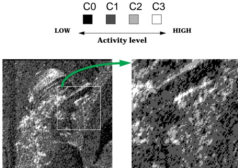
Figure 3.4: 4-level classification map of Subband 8. A causal 6-coefficient context from the same subband is used to obtain the map. Black indicates coefficients from the least active class and white depicts the most active. The right figure, the zoomed detail of the boxed region in the left, shows that classification is performed at the coefficient level.
