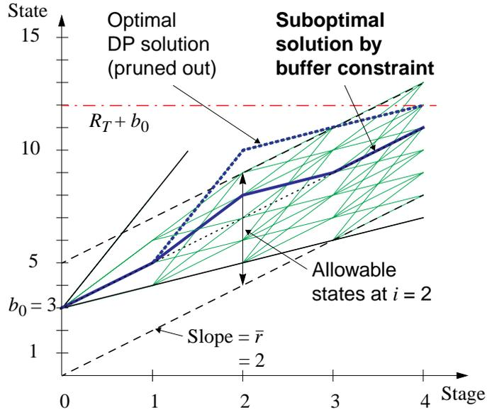
Figure 5.3: Standard DP and buffer-constrained DP. In the standard DP case the number of states grows linearly. By introducing “buffering” constraint, we can keep the number of states at each stage constant. The states are allowed only between the buffer state bounds denoted by the dashed lines. In this example, for the chosen buffer size, the optimal solution cannot be achieved. However note that one could always find a sufficiently large buffer that would not prune out the optimal solution.
