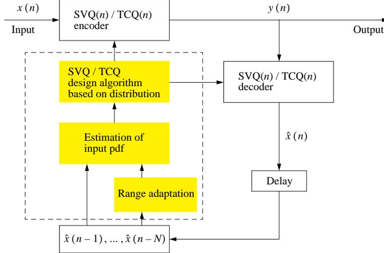
Figure 2.1: Block diagram of backward adaptation. In the diagram, we assume SVQ or TCQ to quantize the input although, in general, we can employ any quantizers for the purpose of actual quantization of input as long as the quantized data can be used to estimate the input distribution.
