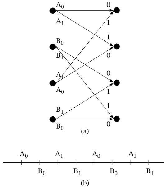
Figure 2.3: 4-state 8-level uniform trellis code. (a) The state transition diagram restricts the quantization of the current input depending on the quantization of the previous input. (b) Quantization levels of the underlying scalar quantizer are partitioned into two sets of  $A = \{A_0, A_1\}$  and  $B = \{B_0, B_1\}$  where each of the subsets  $A_i$ 's and  $B_i$ 's has two corresponding levels.
