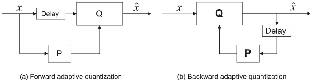
Figure 1.2: Types of adaptive quantization systems. (a) Forward adaptive systems operates based on data to quantize and entails overhead. (b) Backward adaptive quantization operates based on quantized data for adaptation on the fly. No overhead is required but the decoder complexity is increased.
