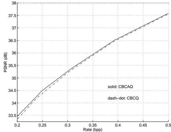
Figure 3.13: Comparison of the image coders with quantizer adaptation and without adaptation, for Lena.
