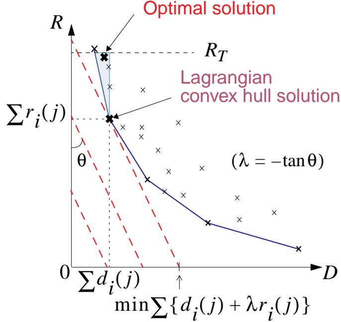
Figure 5.1: Optimal and Lagrangian solutions in the operational R-D space. The convex hull solution is determined as the first point hit by a plane wave of slope  $-1/\lambda$ . The  $D$ -intercept of the plane wave determines the corresponding cost. The shaded area behind the convex hull solution contains the optimal operating point that cannot be reached by this Lagrangian method.
