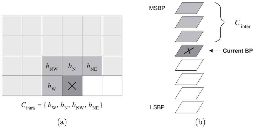
Figure 4.4: Causal contexts to generate the conditional probability model for an input bit to the binary arithmetic coder in IDP. Two sets of bits, (a)  $C_{intra}$  and (b)  $C_{inter}$ , are used to exploit the correlations among neighboring bits within the current bit-plane and across the bit-planes, respectively.
