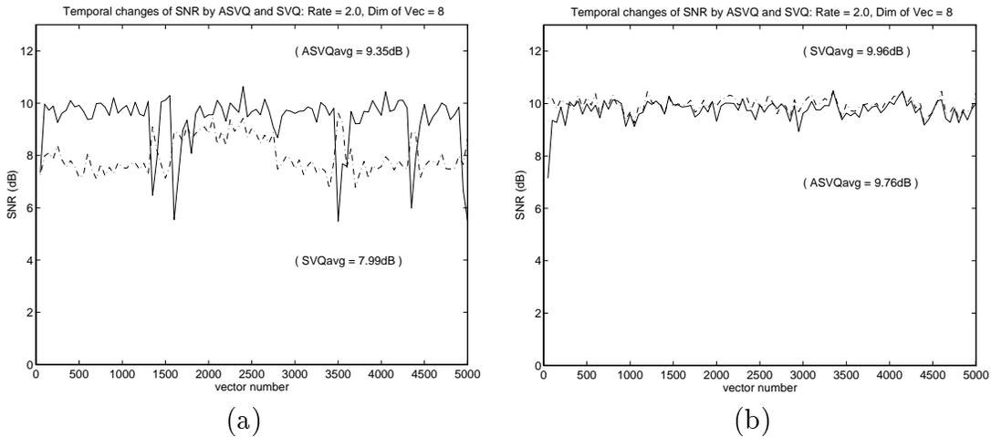
Figure 2.5: ASVQ vs. SVQ (a) When the input is bimodal with each of the modes being Gaussian of the same mean and different variances, the performance of the ASVQ remains nearly constant throughout the sequence except at the point of mode change while SVQ performance is better for one of the two modes. (b) When the input is stationary memoryless Gaussian, there is a slight degradation in performance due to the adaptation.
