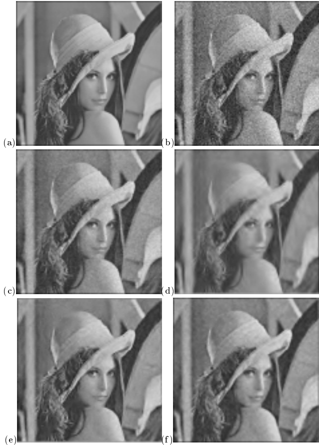
Figure 1: Image denoising using projections onto Besov balls. (a) 512 \times 512 original image with 256 gray levels. (b) Noisy image ( \sigma = 35 , PSNR = 17.2dB). (c) MATLAB's spatially adaptive Wiener filter ( 3 \times 3 window, PSNR = 27.0dB). (d) Hard thresholding in D_{12} domain using threshold chosen to maximize PSNR (PSNR = 26.1dB). (e) Confidence tube denoising algorithm of Ishwar et al. [8] using D_6, D_8, D_{10}, D_{12} and D_{14} (PSNR = 27.5dB). (f) Besov ball projection in B_\infty^1(L_1) using the same 5 wavelet bases (PSNR = 28.3dB).
